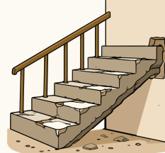
warped, separated, or collapsed staircases
